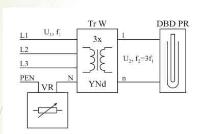
An ozone generator consisted of 12 glass discharge pipes 1.2 m long and with external diameter 90 mm with a capacity of 100 g O3 / h)
