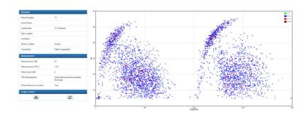
example of internal void PD measured using the TEV sensor.
